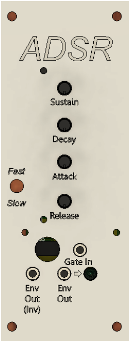
Figure 1.2.3.1: ADSR Panel with Inputs and Outputs
