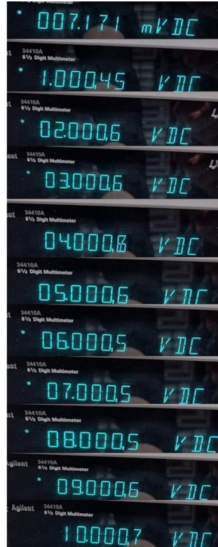
Figure 7.1.2.1: MIDI 2 CV Measurements 0-10V
