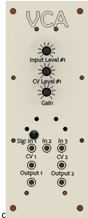
Figure 1.2.4.1: VCA Panel with Inputs and Outputs
